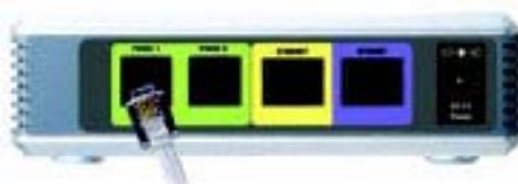
2. Insert the telephone cable into the Phone 1 port of the phone adapter. See figure above.
