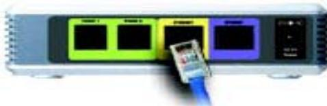
4. Insert the other Ethernet cable into the Internet port and connect the other end into your cable modem.
